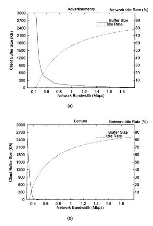
Fig. 9. The optimal network bandwidth, buffer size and network idle rate obtained by our proposed algorithm for (a) *Advertisements* and (b) *Lecture*.
