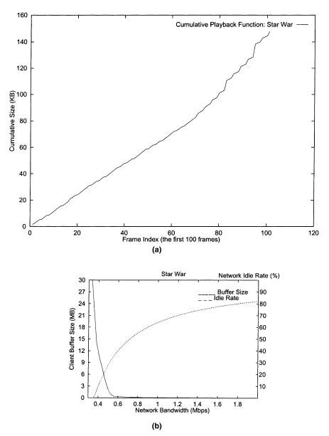
Fig. 7. Star War: (a) The cumulative playback function of the first 100 frames. (b) The optimal network bandwidth, buffer size and network idle rate obtained by our proposed algorithm.
