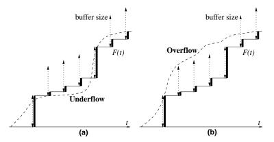
Fig. 2. (a) The underflow (or starvation) condition and (b) the overflow condition for the cumulative transmission function with a bounded client buffer.
