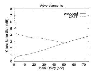
Fig. 11. A comparison of the client buffer size required for our proposed algorithm and CRTT with different initial delay.
