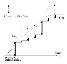
Fig. 1. An example to illustrate the relations among the cumulative transmission function, the cumulative playback function, the initial delay and the client buffer size.
