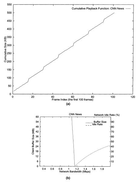
Fig. 8. *CNN News*: (a) The cumulative playback function of the first 100 frames. (b) The optimal network bandwidth, buffer size and network idle rate obtained by our proposed algorithm.
