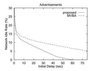
Fig. 12. A comparison of the network idle rate required for our proposed algorithm and MVBA with different initial delay.
