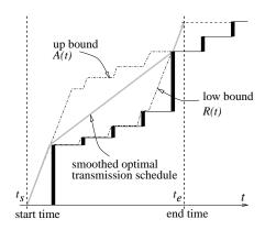
Fig. 5. An example that uses MVBA to the upper bound and the lower bound of the optimal transmission schedules. The result obtained not only has the minimal bandwidth variance but also has the optimal resource allocation and utilization.
