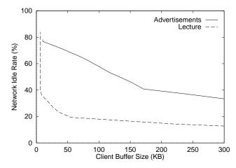
Fig. 10. The relations between the required buffer size and the obtained network idle rate for different streams, *Advertisements* and *Lecture*.
