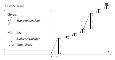
Fig. 3. An example to illustrate the operations of Algorithm-L that minimizes the resource allocation.
